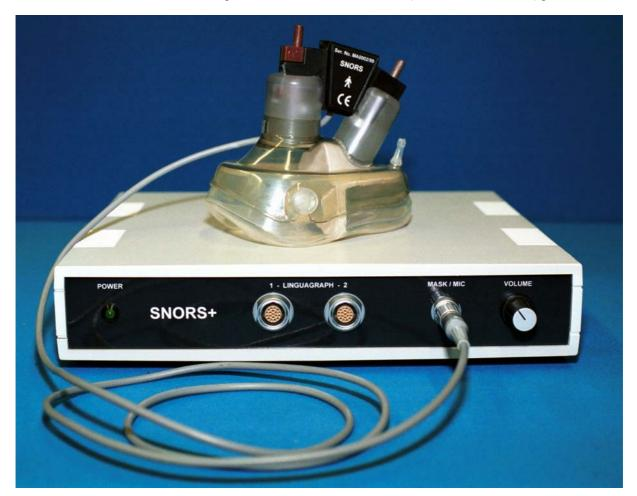
Masks are lightweight and transparent, and both adult and child (4+ years) sizes are available. They are simply held snugly over the nose and mouth by the patient or therapist. The electronics unit has just one adjustment – a volume control, which is easily set to provide a suitable recording level.
